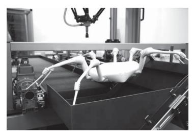
The robot spider's legs are 20 centimeters long. Elastic bellows drives serve as joints. (© Fraunhofer IPA)
