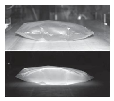
The cell culture bag before (top) and during coating (bottom). (© Fraunhofer IME)
