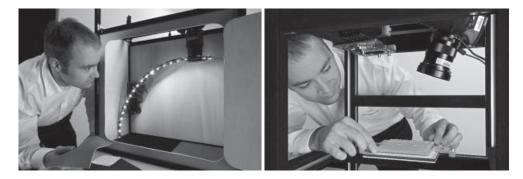
The HDR-ABTF scanner captures physically realistic images of materials such as textiles, lit from various different angles (left). The meso scanner records detailed 3-D structures of surfaces with great precision (right). (© Fraunhofer IGD)
