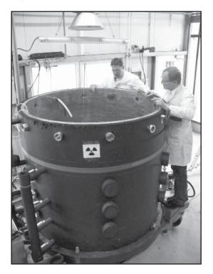
Researchers inspect the two-cubic-meter water tanks equipped with a powerful filter system. (© Fraunhofer IME)
